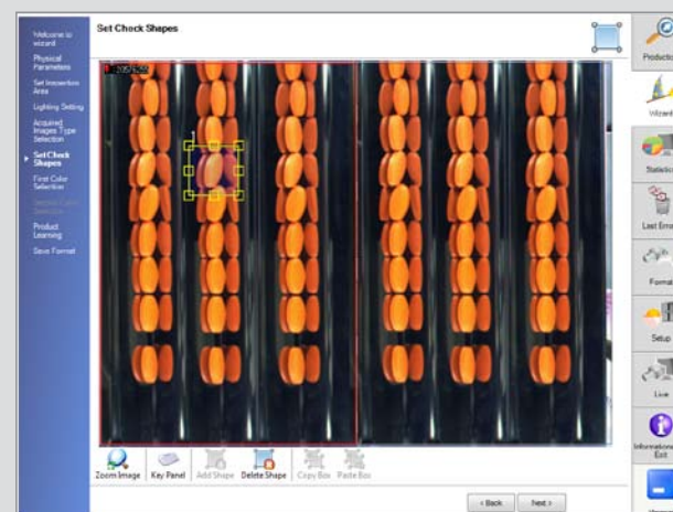
WIZARD PROCEDURE FOR CHECK REGION POSITIONING
